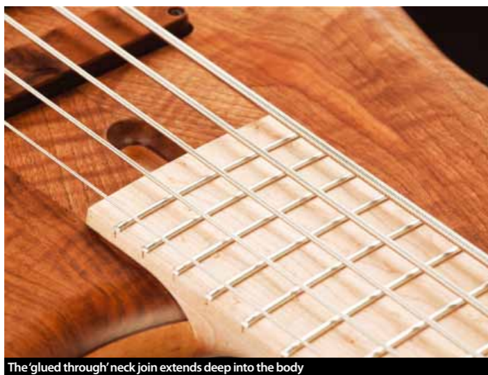
The 'glued through' neck joint extends deep into the body
